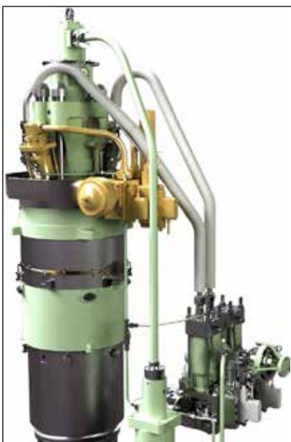
This block contains a control valve for methanol fuel injection, a sealing booster activation valve, a forced suction activation valve, an LGI purge valve and methanol fuel inlet/outlet valves. All pipes for hydraulic oil and fuel are double-walled. Furthermore, the double-walled pipes for methanol fuel are vented with ventilation air, see Fig. 2.
